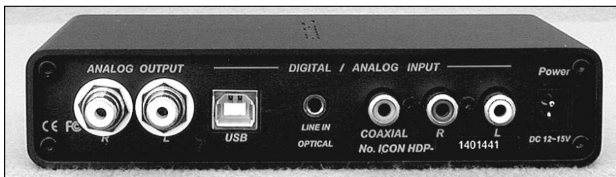
PHOTO 2: The rear panel of the HDP includes analog input and output jacks, USB, S/PDIF and optical digital inputs, and the power supply connector.
