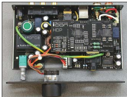
PHOTO 4: The Icon HDP circuitry is housed on two circuit boards, with the smaller digital board piggybacked onto the main analog board. The volume control and selector switch are high-quality parts.
