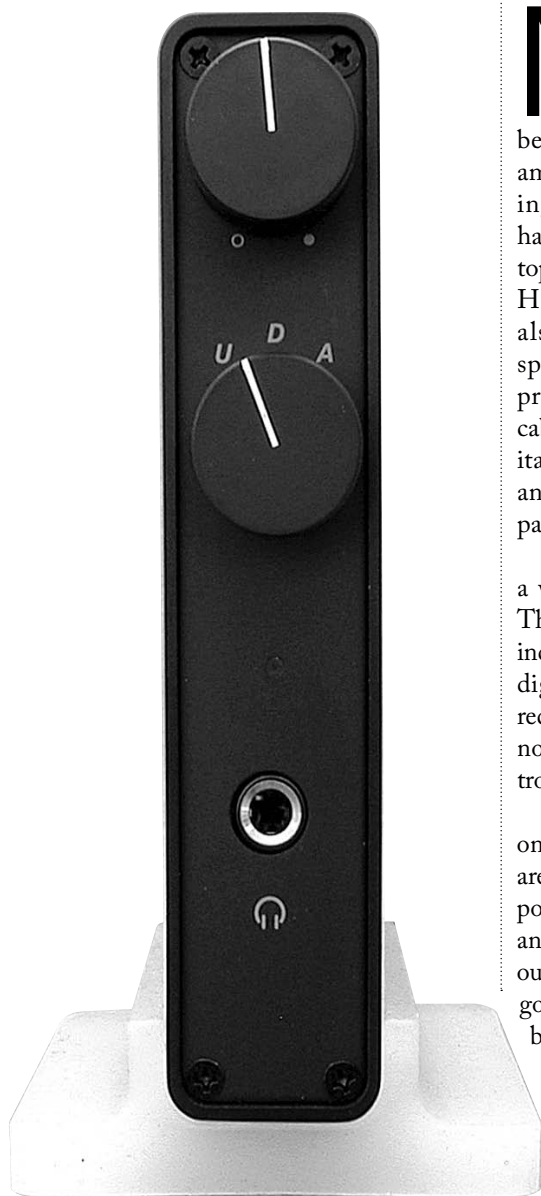
PHOTO 1: The front panel of the NuForce Icon HDP contains a volume control, input selector, and a 1/4" stereo headphone jack.
